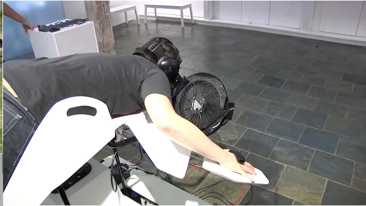
Birdly (Zürich University of Art and Design) Types of feedback: visual, auditory, haptic, wind, smell
